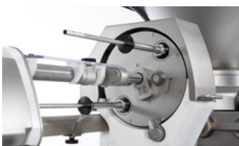
↑ Casing spooling with semi-automatic casing change function
