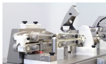
↑ Precise separating with 2-belt solution and sensor
